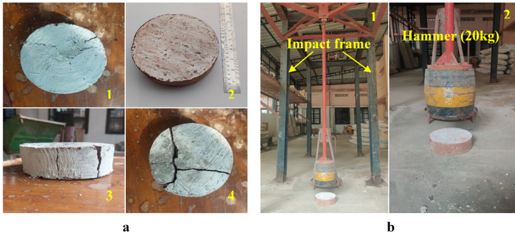
Fig. S6. Impact resistance of EGC mixes (a) test specimens (b) impact test setup
